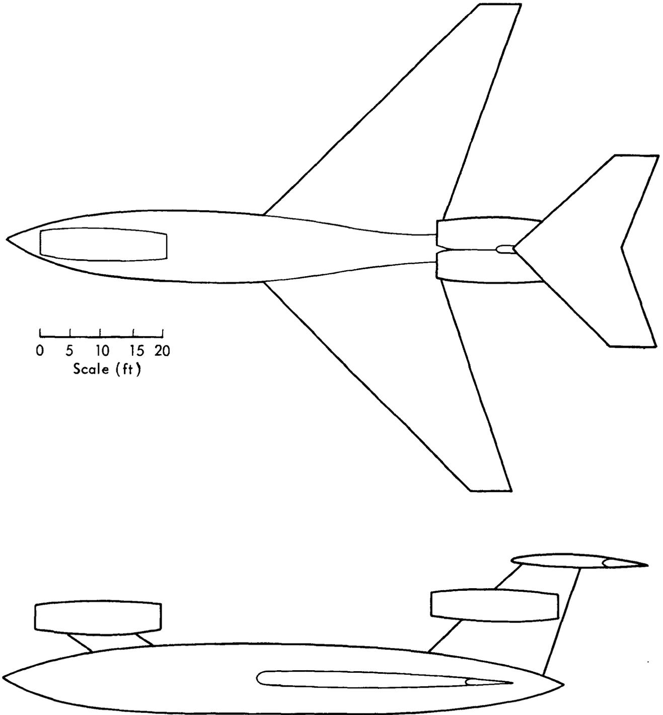
Fig. 13—Submersibly moored shuttle tanker of high-tensile steel
