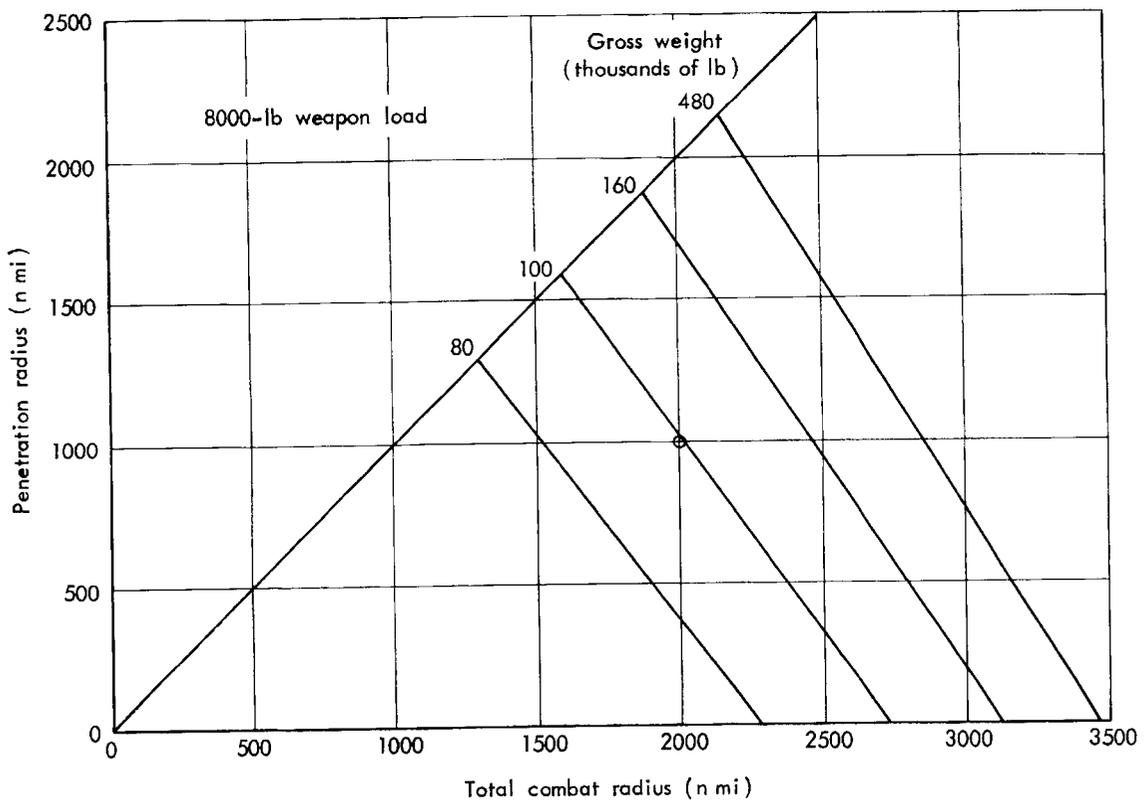
Fig. 3—Combat-radius capabilities of a class of subsonic, submersible penetrator aircraft (submersibly moored, high-tensile-steel construction, aspect ratio 4, JP-4 fuel)
