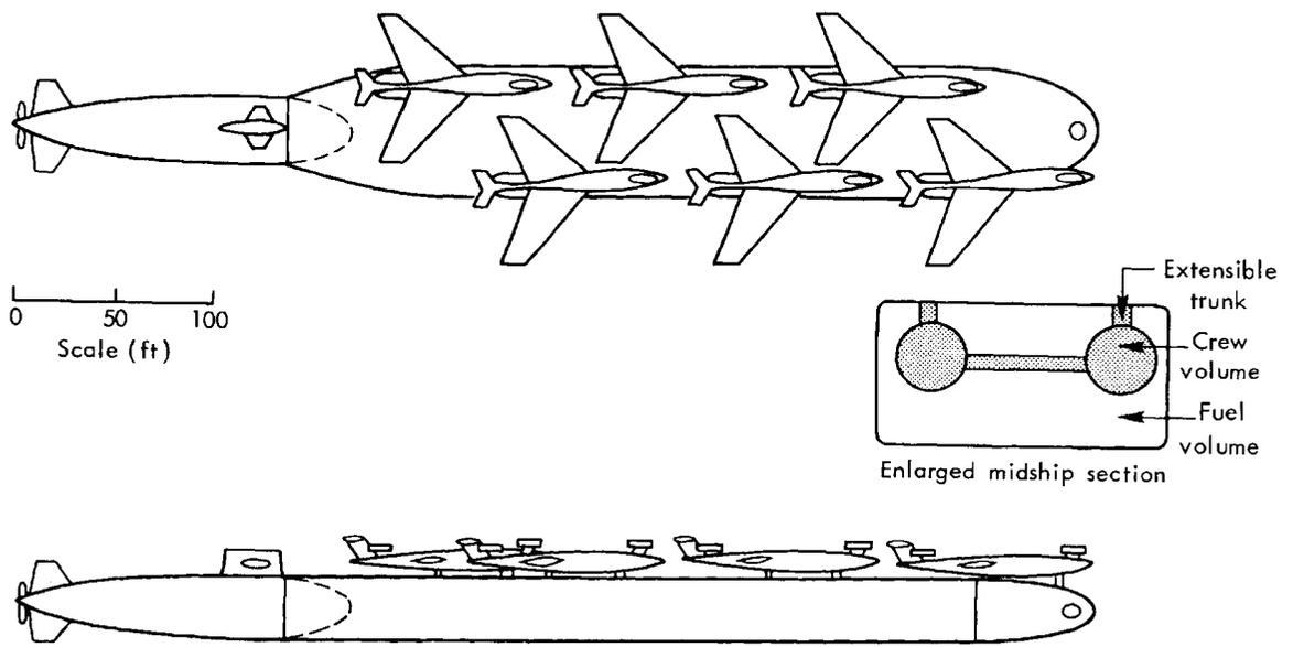
Fig. 16—Submersible tanker-aircraft platform with nuclear pusher tug and complement of six aircraft
