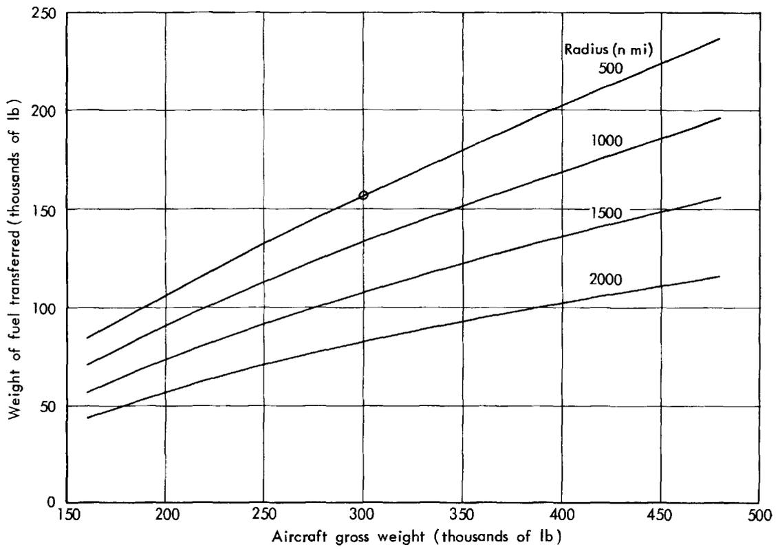
Fig. 15—Fuel-transfer capability of submersible tanker aircraft (submersibly moored, high-tensile-steel construction, aspect ratio 4, JP-4 fuel)
