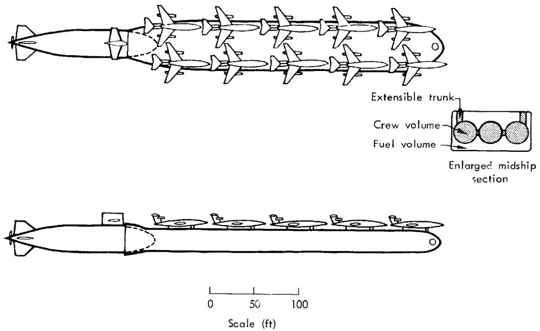
Fig. 4—Submersible penetrator aircraft platform with nuclear pusher tug and complement of ten aircraft
