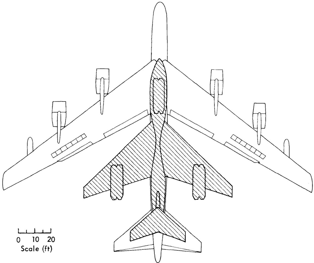
Fig. 1—Size comparison of high-density, highly loaded submersible aircraft with B-52 (equal gross weights)
