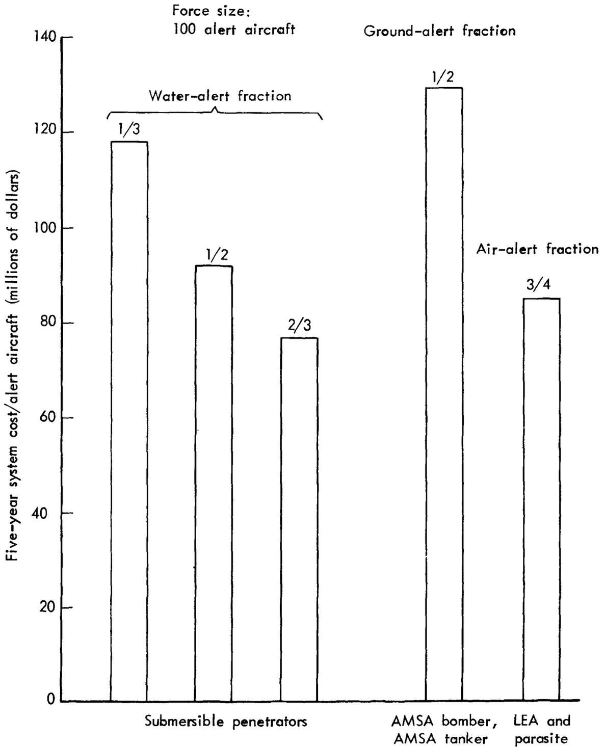
Fig. 5—System costs per alert penetrator aircraft with alternative supporting systems (submersible penetrators affixed for deployment and alert—low mobility)
