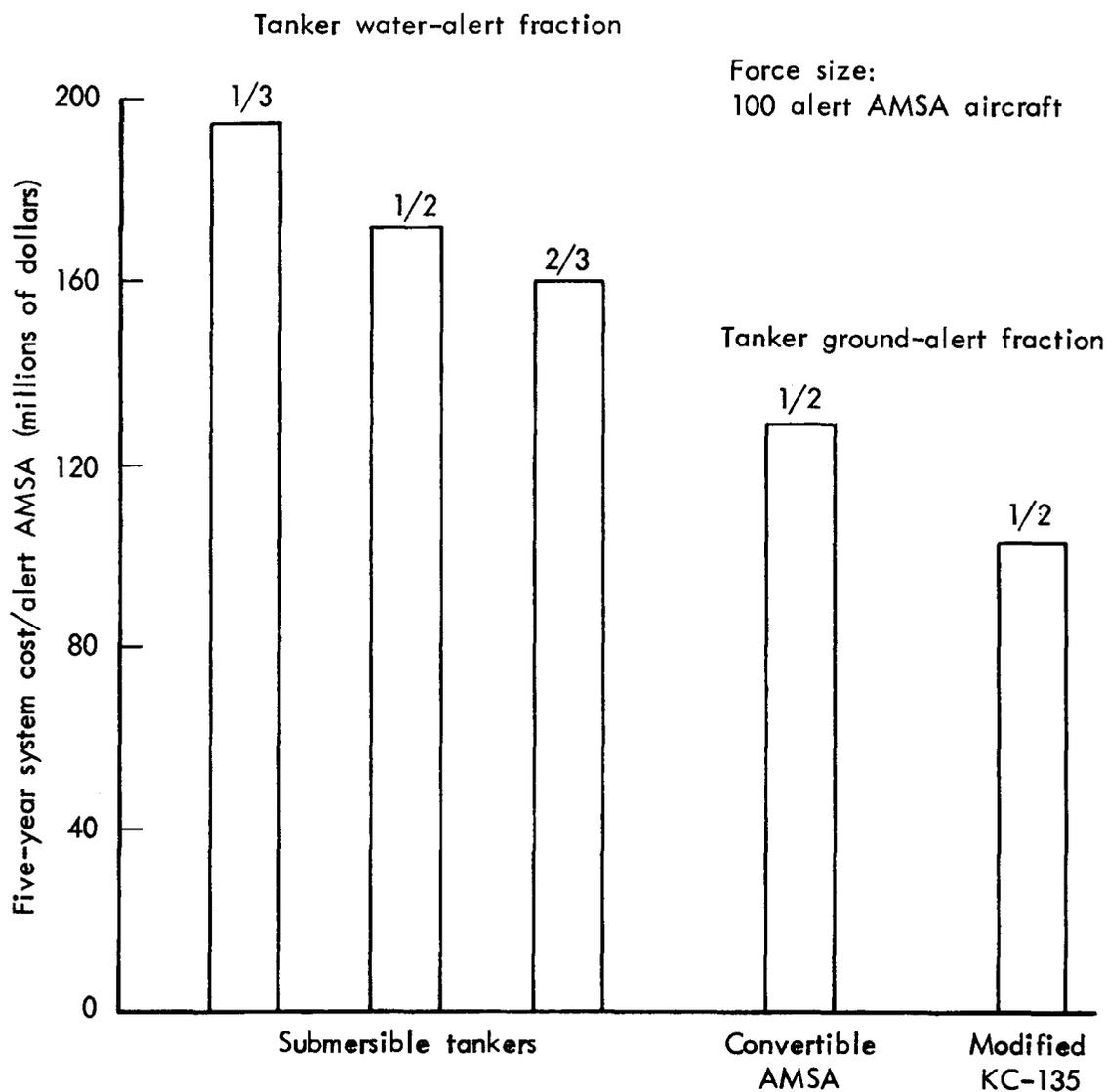
Fig. 17—System costs per alert AMSA with alternative supporting tankers (submersible tankers affixed for deployment and alert—low mobility)
