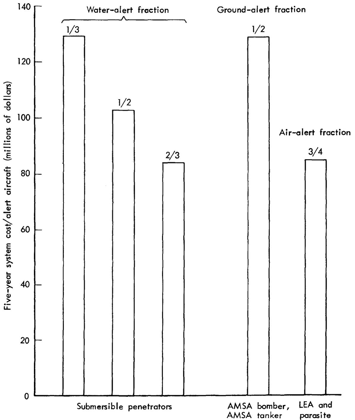
Fig. 7—System costs per alert penetrator aircraft with alternative supporting systems (submersible penetrators affixed for deployment but on individual alert—high mobility)
