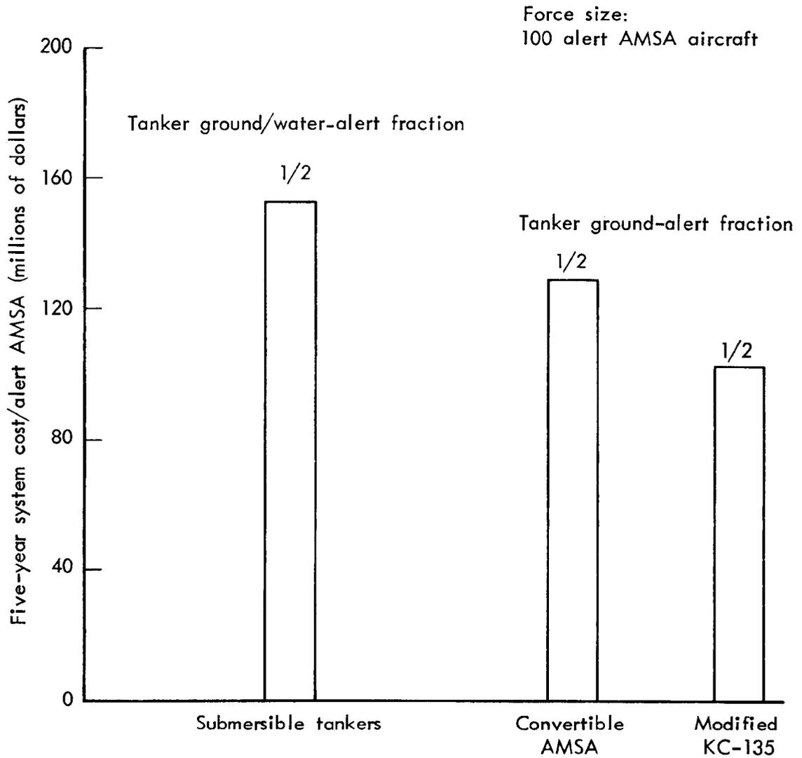
Fig. 18—System costs per alert AMSA with alternative supporting tankers (submersible tankers flown forward for individual alert—land-based flyout)
