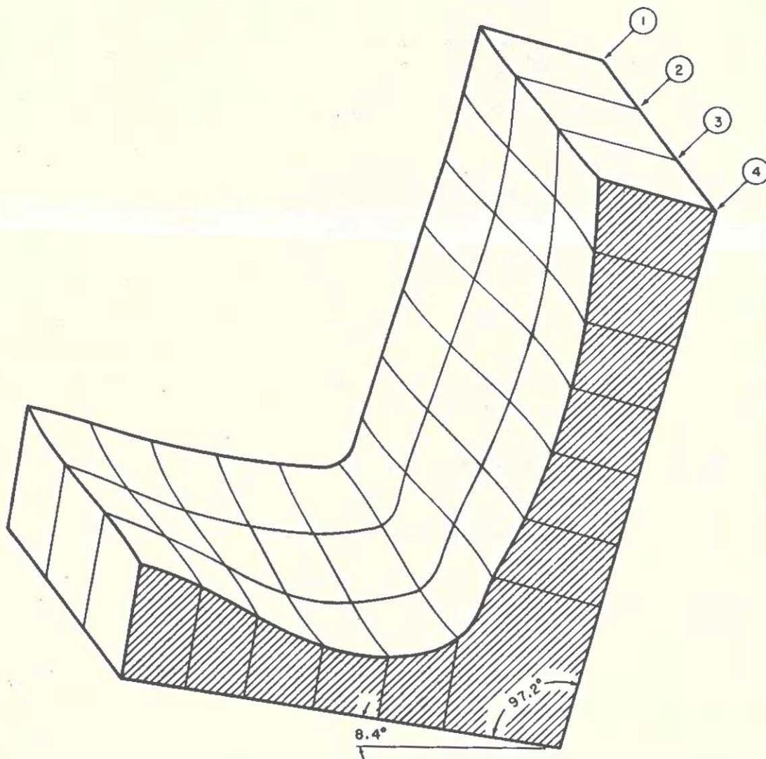
SEAT SECTION FOR 41" BOMBER COCKPIT, SHOWING PROFILES AT  $\frac{1}{2}$  (4) AND
