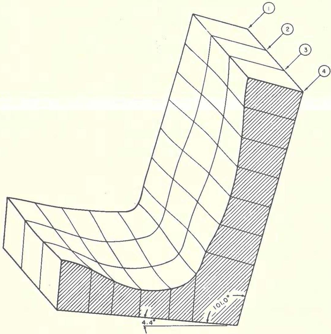
SEAT SECTION FOR 45" BOMBER COCKPIT, SHOWING PROFILES AT  $\xi$  (4) AND AT
